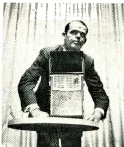
Two-in. picture tube gives 80-sq-in. display (left) in new set using 21 transistors and a battery rechargeable through outlet (right)
