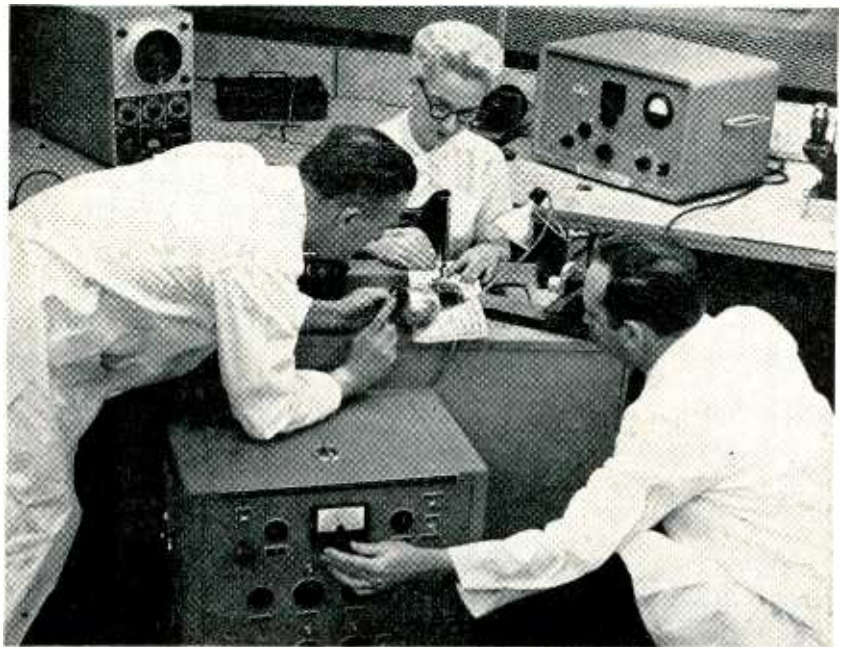
Operator at right adjusts controls of strobe analyzer prior to taking series of photos of a malfunctioning sewing machine attachment; photos taken at millisecond intervals, will point to corrective action
