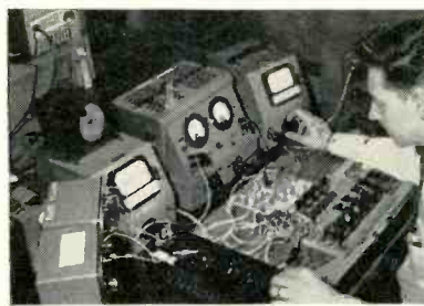
Setup used to prepare matched sets of transistors
