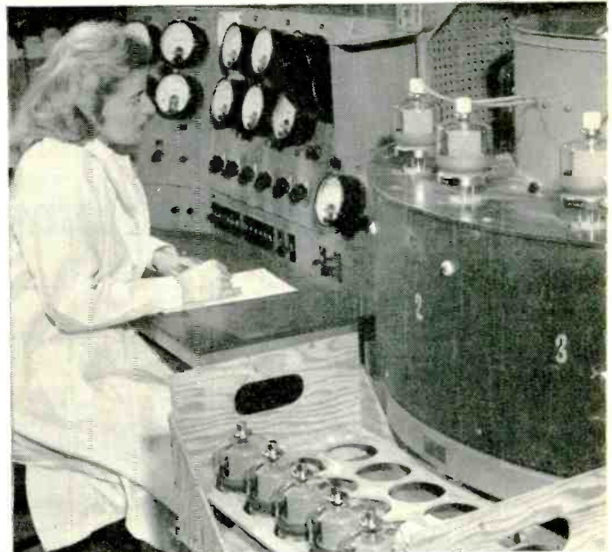
Every tube meets rigid Eimac specifications before shipment. On test consoles like this, dozens of electrical characteristics are patiently tested and recorded for each Eimac tube produced. Environmental testing equipment is also available for testing for severe applications.
