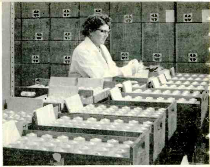
Ready for shipment, these Eimac ceramic tetrodes are just one of more than a hundred different tube types manufactured by Eitel-McCullough, Inc., including negative grid tubes, power amplifier klystrons, reflex klystrons and traveling wave tubes.
