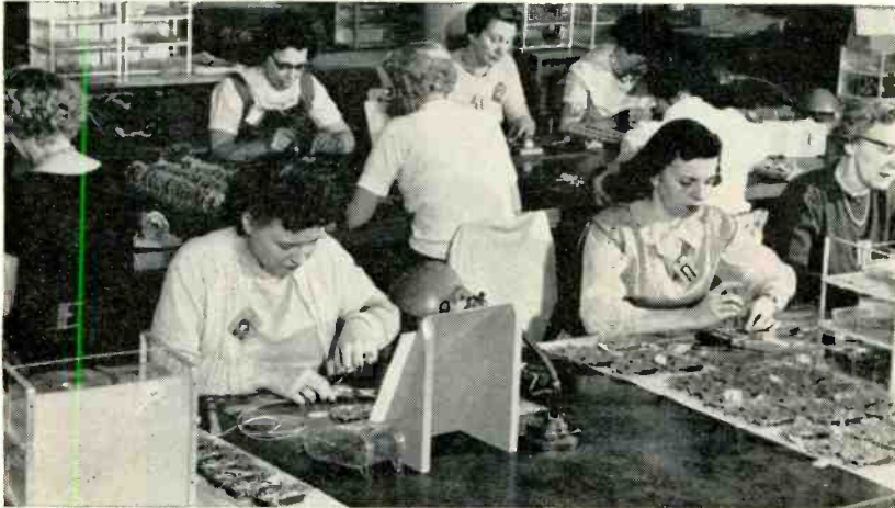
Portion of village. Each assembler spends the same amount of time on a board, passes work to girl on left
