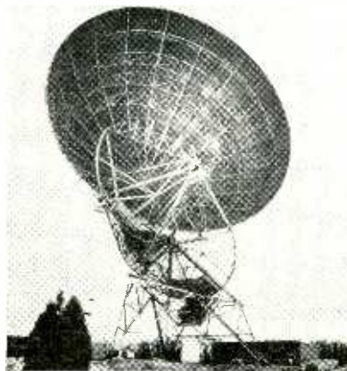
New 85-ft radio telescope at University of Michigan receives wave lengths as short as 3 cm. Projects planned include study of 21-cm radiation from our galaxy and other galaxies
