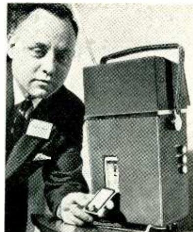
Two-in. picture tube gives 80-sq-in. display (left) in new set using 21 transistors and a battery rechargeable through outlet (right)
